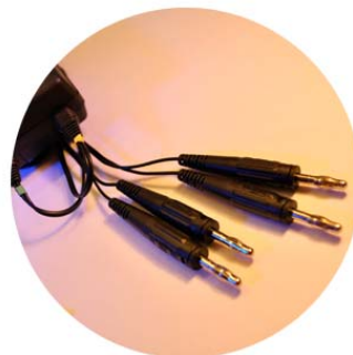
Twin leads showing their four connectors
