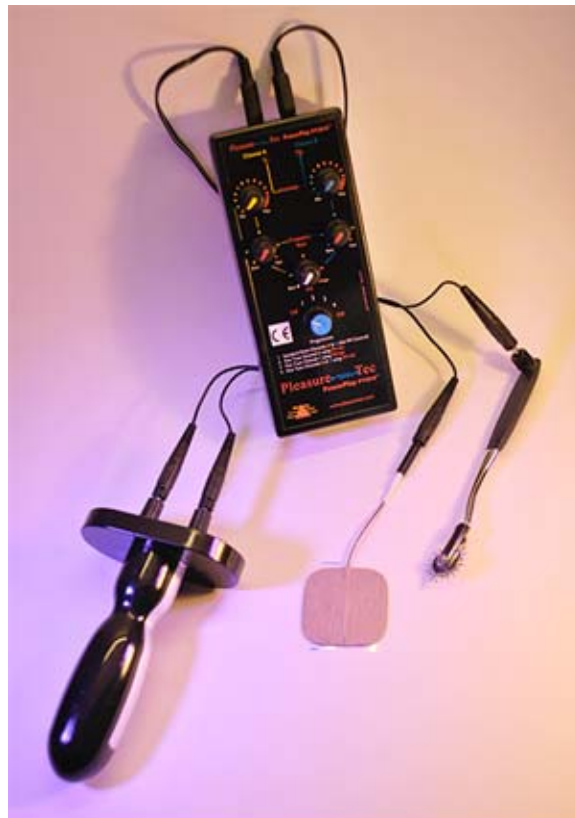
This shows two channels being used. One with a Bi-Polar item, one with two Uni-Pole items.
